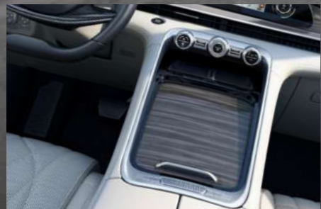
Armrest Box with Refrigeration and Heating
